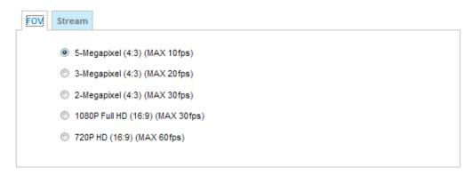
Select a resolution from the list. The default is 5 Megapixels, and if bandwidth or frame rate per second is of the concern you can select a lower resolution. The configurable options are: 5MP (4:3) at 10fps, 3MP (4:3) 20fps, 2MP (4:3) 30fps, 1080P (16:9) 30fps, and 720P (16:9) at 60fps.
